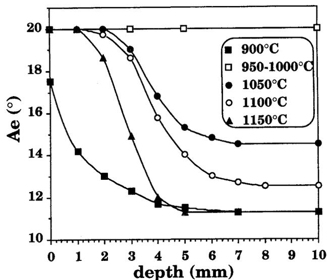
Fig. 3 Pyrocarbon texture profiles ( $A_e$ ) along the 60  $\mu\text{m}$  model pore as a function of  $T$  ( $t_R=10\text{ s}$  and  $P=3\text{ kPa}$ ).
