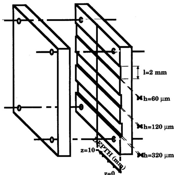
Fig. 1 Schematic of the model pores.
