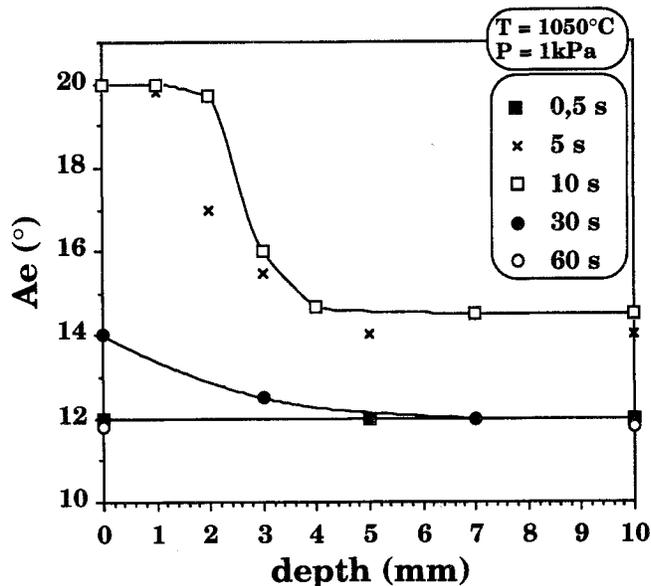
Fig. 2 Pyrocarbon texture profiles ( $A_e$ ) along the 60  $\mu\text{m}$  model pore as a function of  $t_R$  at  $P = 1\text{ kPa}$ .
