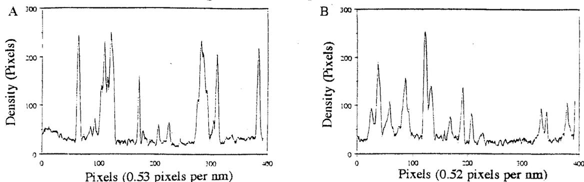
Figure 2. Density plots generated from scans of 002 dark-field images of (A) Fiber A and (B) Fiber B.
