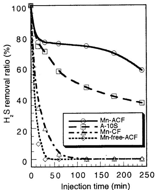
Figure 1 - H<sub>2</sub>S removal abilities of the fibers prepared.
