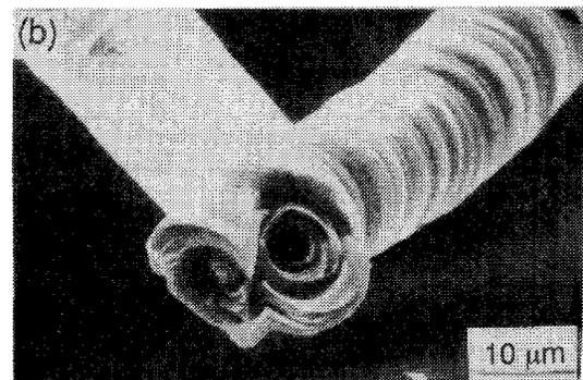
Fig.1 (a) Morphology of vapor-grown carbon fibers and (b) structure of a branching point.
