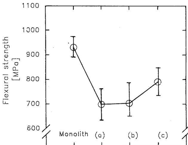
Fig. 1. Comparison of flexural strength of ceramics composites with carbon fibers.
