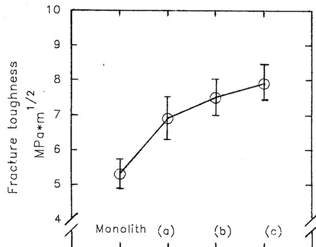
Fig. 2. Comparison of fracture toughness of ceramics composites various carbon fibers.
