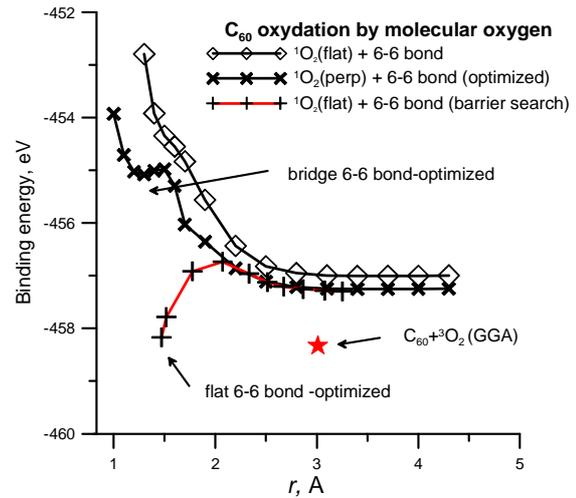
Fig. 1 DFT PES of the atomic/molecular oxygen near a C<sub>60</sub> molecule..
