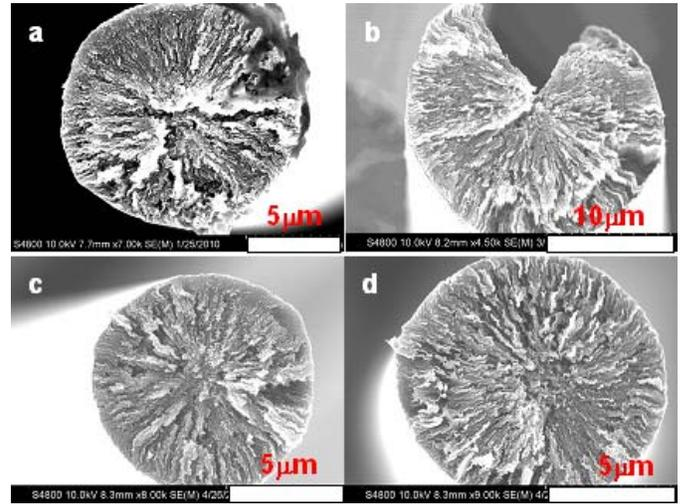
**Fig. 1** SEM micrographs of carbon fibers being heat treated at 2500°C: a. L<sub>1</sub> (806), b. L<sub>1</sub>S<sub>1</sub> (680), c. L<sub>2</sub> (444), and d. S<sub>1</sub> (443).
