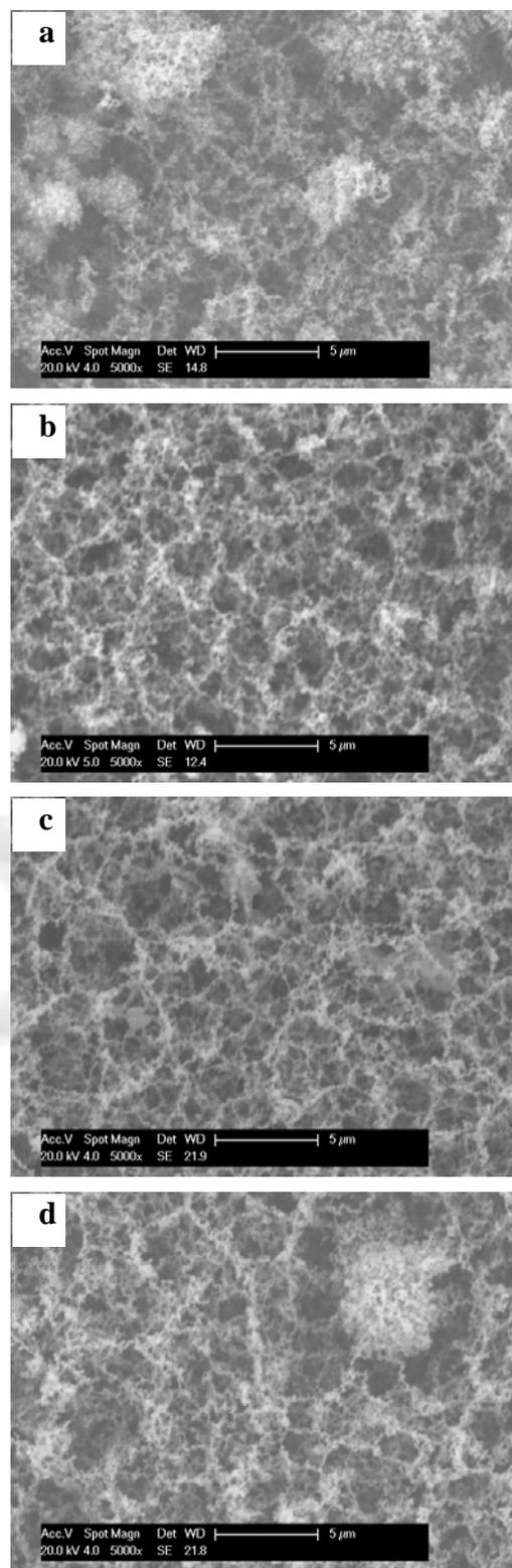
**Fig. 2** SEM images of the carbon films obtained when the SSS was put at one side ((a) and (c)) of or under ((b) and (d)) the ADR, with the carbon black ((a) and (b)) and graphite ((c) and (d)) as carbon source, respectively. The nitrogen temperature was 800 °C.
