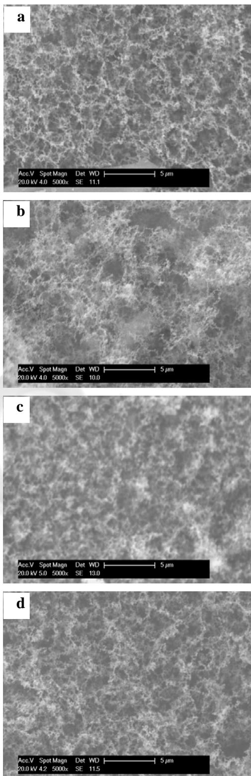
**Fig. 1** SEM images of the carbon films obtained at (a) and (c) room temperature, (b) and (d) 800 °C of nitrogen, with the carbon black ((a) and (b)) and graphite ((c) and (d)) as carbon source, respectively. The SSS was put above the ADR.
