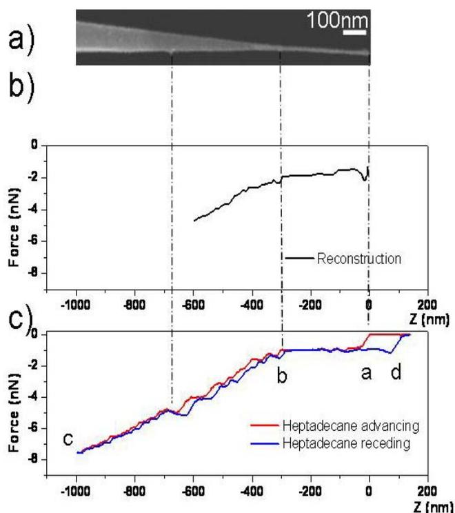
**Fig. 1** a) FEG-SEM micrograph of one of the carbon-cone tip used as a capillary force probe. The far tip (on the right) is cylindrical because it corresponds to the nanotube used to deposit the carbon cone onto it. b) Reconstruction of the theoretical force applied on the probe. c) Capillary force measurement (red: dipping-in, and blue: dipping-out) in heptadecane.
