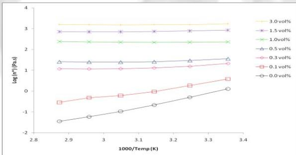
**Fig4.** The complex viscosity  $n^*$ (Pa·s) vs. 1000/Temperature (K) at  $\omega = 10$  rad/s for loadings of 0, 0.1, 0.3, 0.5, 1.0, 1.5, and 3.0 vol % MWCNTs in epoxy
