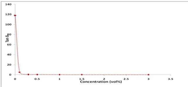
**Fig 3.**  $\tan \delta$  vs. MWCNT Concentration (vol %) at  $\omega = 10$  rad/s & 25°C
