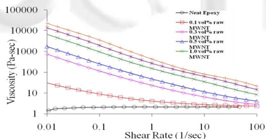
**Fig 1.** Viscosity measured as function of decreasing shear rate
