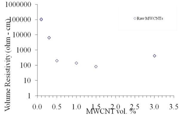
**Fig 5.** Resistivity of Epoxy- raw MWNT Composites
