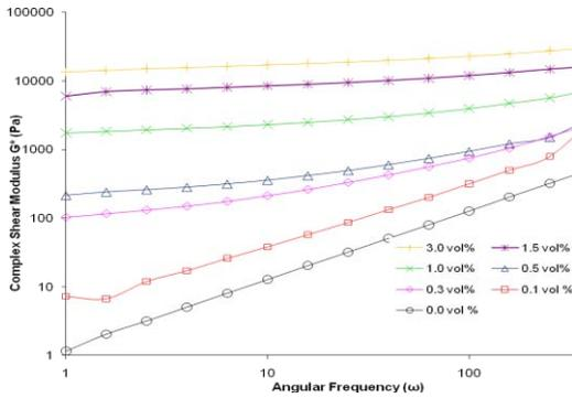
**Fig 2.** Modulus ( $G^*$ ) vs. Angular Frequency ( $\omega$ ) at 25°C for all loadings.
