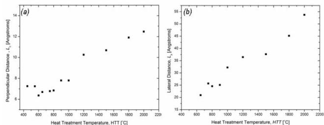
**Fig. 2.** Calculated (a) crystalline thickness,  $L_c$  and (b) lateral distances,  $L_a$ .
