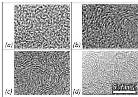
**Fig. 3** HR-TEM images of microcrystalline cellulose samples heat treated to (a) 250°C, (b) 600°C, (c) 1000°C, and (d) 2000°C.
