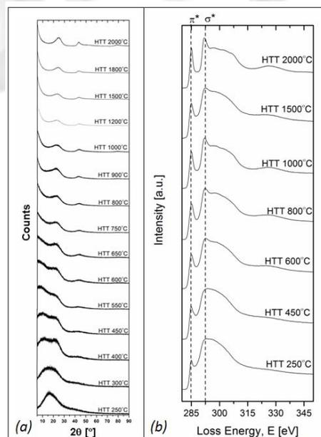
**Fig. 1** (a) XRD patterns and (b) EELS spectra for heat treated microcrystalline cellulose.
