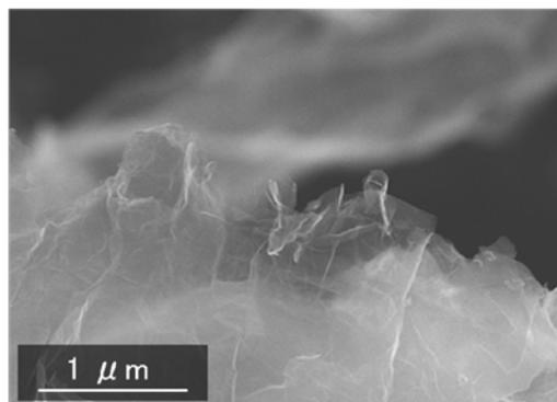
Fig. 1 Exfoliated graphite particles
