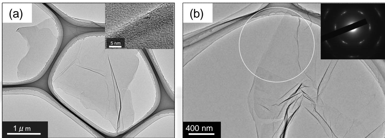
Fig. 2 TEM micrographs of (a) graphene-like carbon thin layers (b) SAED pattern on its carbon thin layers.
