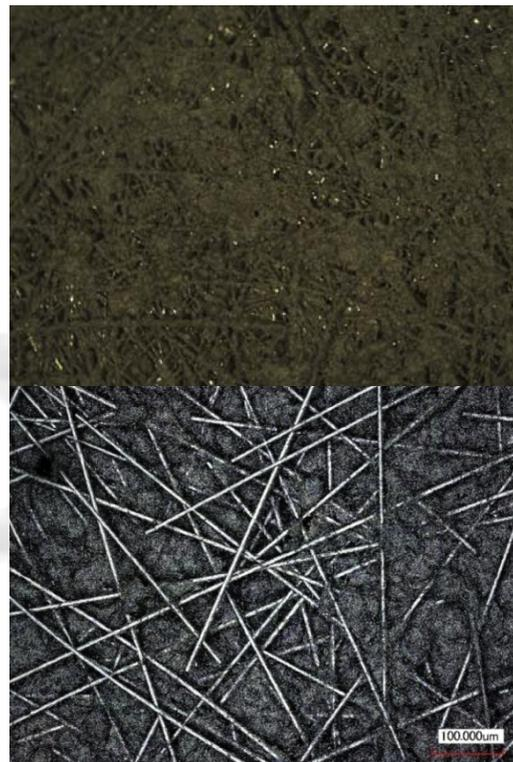
**Fig. 1** Optical images of nanofiber mat produced via spraying. The spray process generates a well-developed network of nanofiber supported by the carbon fiber veil.
