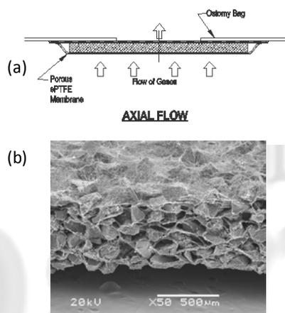
**FIG. 1** Cross-sectional view of the filter assembly adhered to an ostomy bag (a) axial flow (b) SEM image of a filter assembly described in FIG. 1a.
