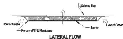
**FIG. 2** Cross-sectional view of the filter assembly adhered to an ostomy bag: lateral flow.
