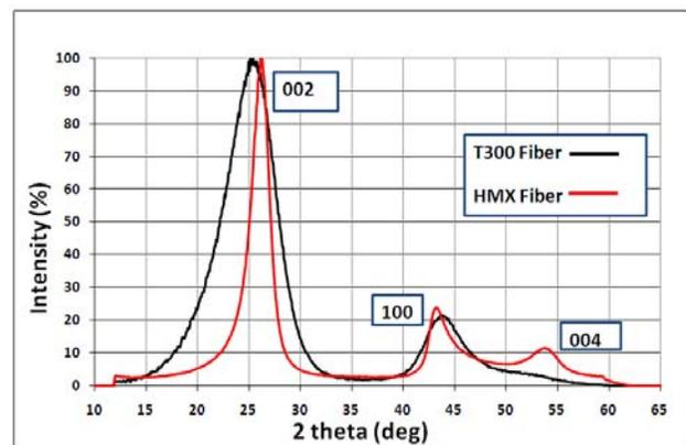
**Fig 1.** WAXD 2 theta scan curves of T300 fiber and an experimental high modulus (60 msi) fiber
