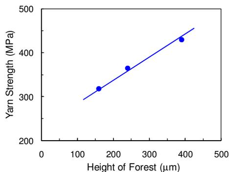
**Fig.1** Dependence of the strength of a twist-spun MWNT yarn on the height of the MWNT forests.
