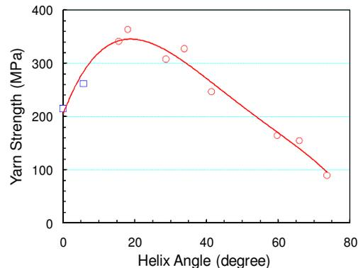
**Fig. 2** Dependence of yarn tensile strength on yarn helix angle for forest spun MWNT yarn. Yarns having very low twist (squares) were liquid densified before twist insertion, and the remaining yarns (circles) were twist spun without any prior treatment. The yarn diameter was kept constant at  $\sim 20$  μm.
