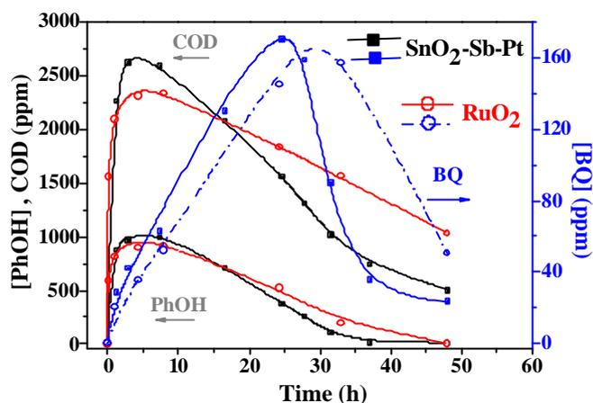
**Fig. 1** Evolution of phenol (PhOH), COD and p-benzoquinone (BQ) in the NaOH electrolyte during regeneration experiments performed with different anodes ( $I = 0.5 \text{ A}$ ; Total time = 48 h).
