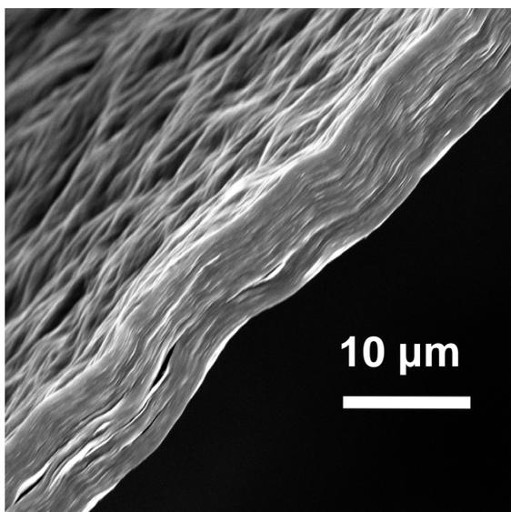
**Fig. 1** SEM image of graphene paper.
