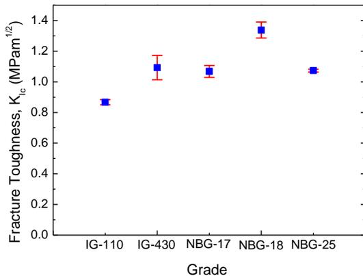
**Fig. 2** Fracture toughness,  $K_{Ic}$  of nuclear grade graphite.
