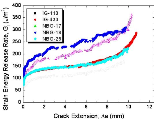
**Fig. 3** Strain energy release rate,  $G_I$  of nuclear grade graphite
