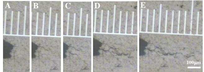
**Fig. 1** Typical load-displacement curve for IG-110 and microcracks formation in the notch tip.
