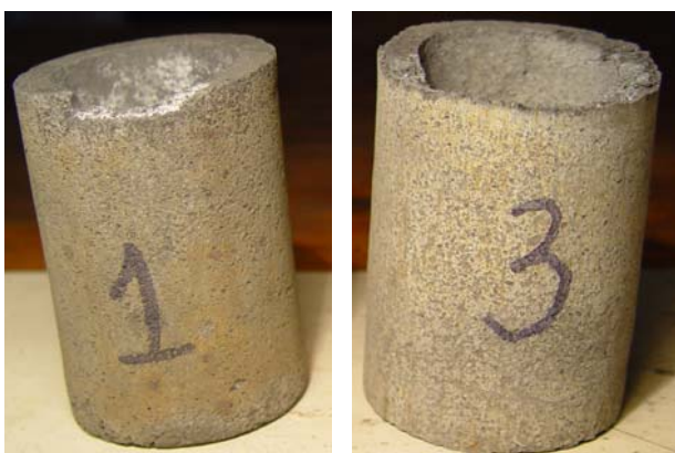
Fig.3 Experimental carbonaceous metalcarbide crucibles during testing.
