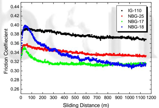
**Fig. 2** Variation of friction coefficient with sliding distance
