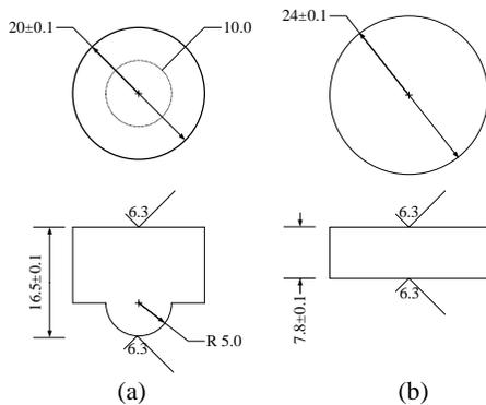
**Fig. 1** Ball-on-disk type wear specimens; (a) upper and (b) lower specimens.
