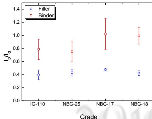
**Fig. 4** Raman peak ratio,  $I_D/I_G$  in the filler and binder phases
