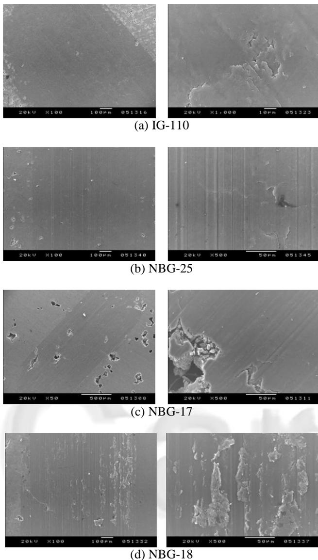
**Fig. 3** SEM photos of worn surfaces
