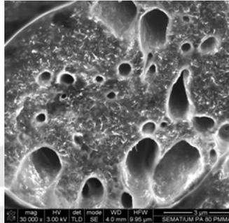
Fig. 1 SEM micrographs of the cryo-fractured cross sections of the filament composites after dissolution of PMMA phase.
