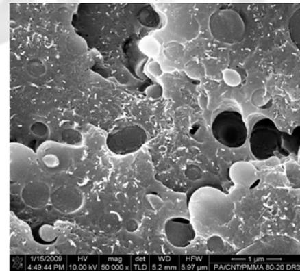
Fig. 2 SEM micrographs of the cross sections of PA12 / PMMA (A), PMMA(18%)/CNT (4%)/PA12 (78%) (B), and PA12(78%)/CNT (4%)/PMMA (18%) (C).
