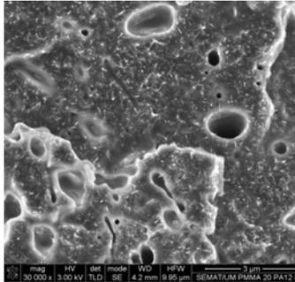
PA12(78%) / CNT (4%) / PMMA (18%)
