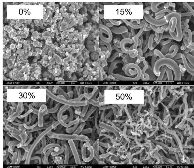
**Fig. 2** SEM images of as-prepared products at different CO<sub>2</sub> concentrations operated at 560 °C over unsupported Fe catalyst.
