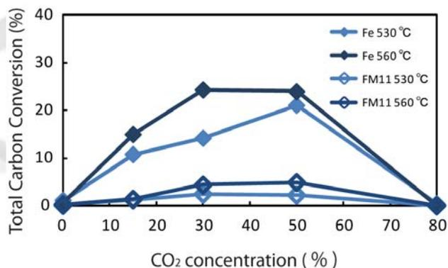
**Fig. 1** Total carbon conversion at CO<sub>2</sub> concentration between 0% and 80% for unsupported or MgO-supported Fe catalysts at 530 °C and 560 °C
