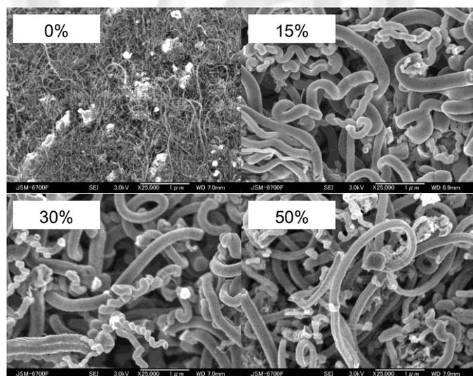
**Fig. 3** SEM images of as-prepared products at different CO<sub>2</sub> concentrations operated at 560 °C over MgO-supported Fe catalyst.
