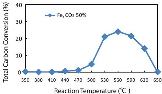
**Fig. 4** Total carbon conversion at 50 % of CO<sub>2</sub> concentration using Fe catalyst at different growth temperatures
