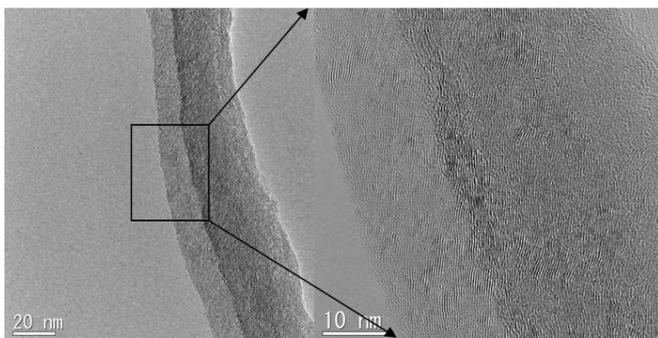
**Fig. 3** Detailed TEM observation of CNFs produced over Fe-Mn (3/7) catalyst at 540 °C
