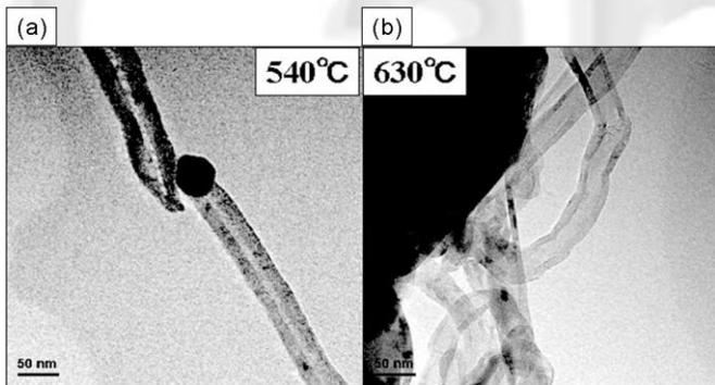
**Fig. 2** TEM photographs of CNFs produced over Fe-Mn (3/7) catalyst at 540 °C and 630 °C.
