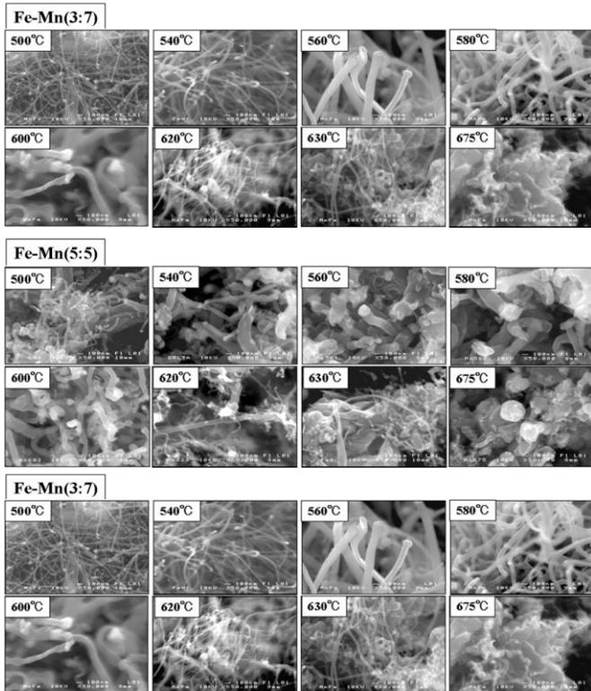
**Fig. 1** SEM photographs of CNFs produced for CO/H<sub>2</sub> mixture of 1/4 over Fe-Mn (7/3) catalyst in a temperature range of 500 to 675 °C
