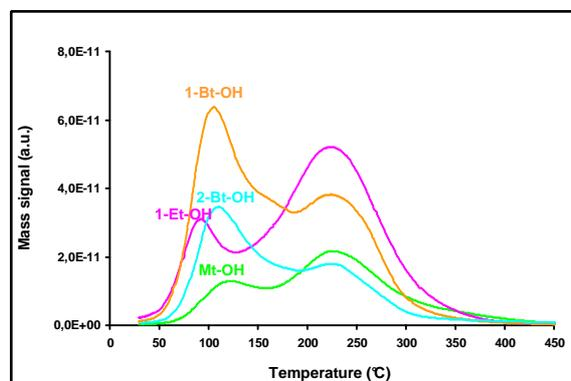
**Fig. 2** TPD desorption profile for different type of alcohols (a) methanol (b) ethanol (c) 1-butanol and (b) 2-butanol adsorbed on carbon surface from their mixture with cyclohexane.
