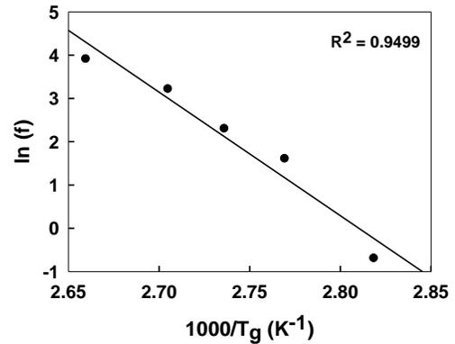
**Fig. 4** Relation between  $f$  and  $T_{gt}$ ;  $f$ : test frequency, and  $T_{gt}$  was measured by tan delta.
