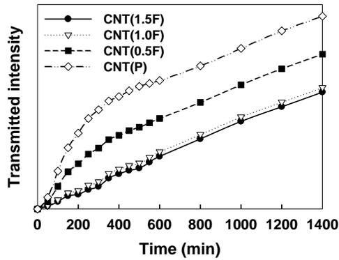
**Fig. 1** Effects of fluorination on MWCNTs based on their dispersion in epoxy resin blend.
