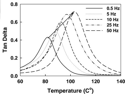
**Fig. 3** Tan delta of EC(1.0F) at a heating rate of 2 °C/min and at various frequencies.
