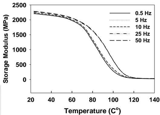
**Fig. 2** Storage modulus of EC(1.0F) at heating rate of 2 °C/min and various frequencies.
