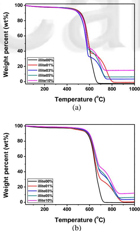
**Fig. 2** TGA results of the C/C composites with various illite contents prepared at (a) 1000 °C and (b) 1650 °C.
