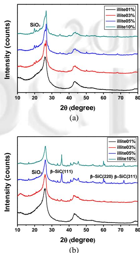
**Fig. 1** XRD patterns of illite/phenol composites carbonized at (a) 1000 °C and (b) 1650 °C.
