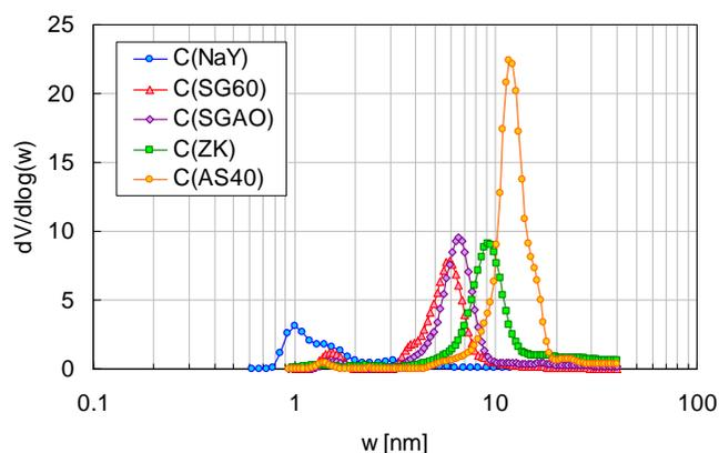
**Fig. 1** Pore size distributions for nanostructured carbons.
