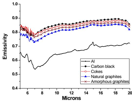
Fig. 2. Emissivity curves of coated powders at 50 °C.
