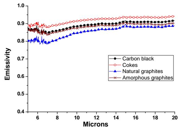
Fig 1 Emissivity curves of raw powders at 50 °C.
