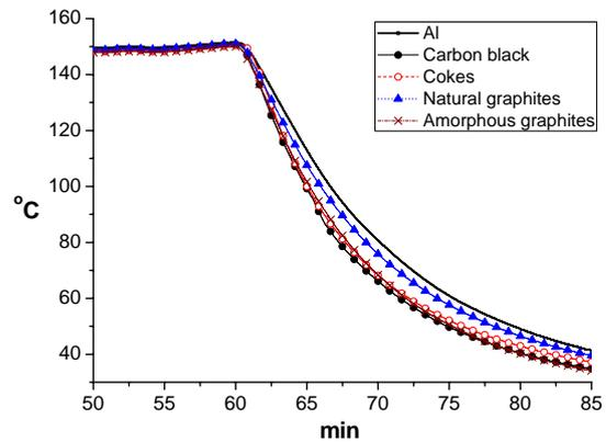
Fig. 3. Comparison of cooling rate as a function of coating condition.
