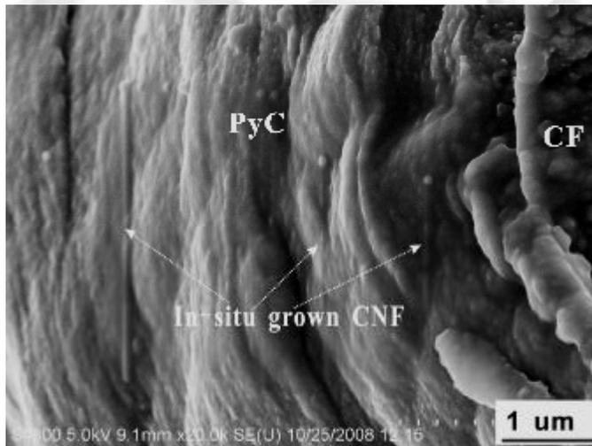
**Fig.3** In-situ grown CNFs in pyrolytic carbon during chemical vapor infiltration processing
