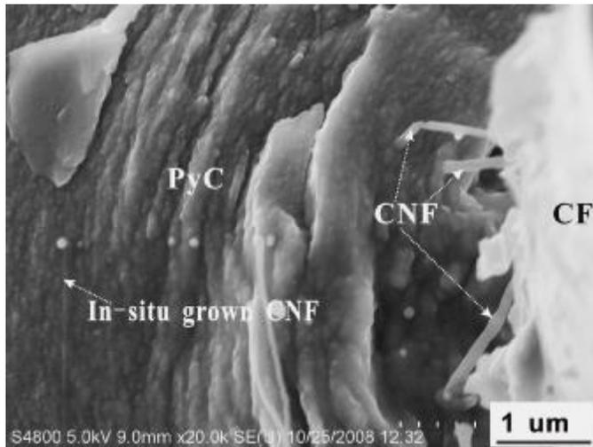
**Fig.2** CNF bridge-combinations between carbon fiber and the surrounded pyrolytic carbon matrix
