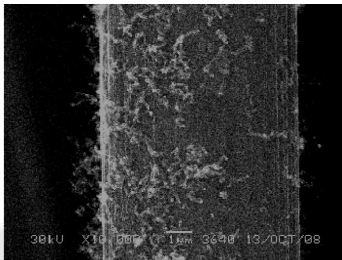
Fig.1 SEM image of the carbon fibers with carbon nanofibers
