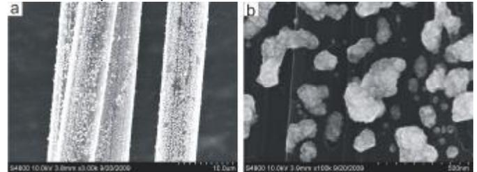
Fig.1 Morphology of Ni catalysts on carbon fibers.
