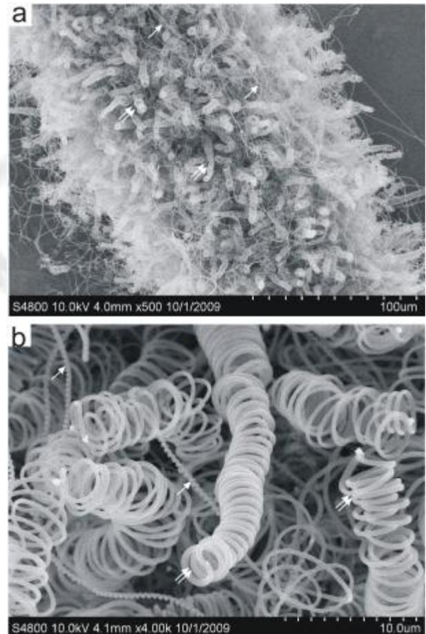
Fig.2 SEM images of carbon microcoils grown on PAN-based carbon fibers. (a) the overall morphology of a carbon fiber with carbon microcoils grown on; (b) magnified view of typical carbon microcoils in (a). Noted: the white single arrows shows twisting single-helix coils and the white double ones shows spring-like double-helix microcoils.
