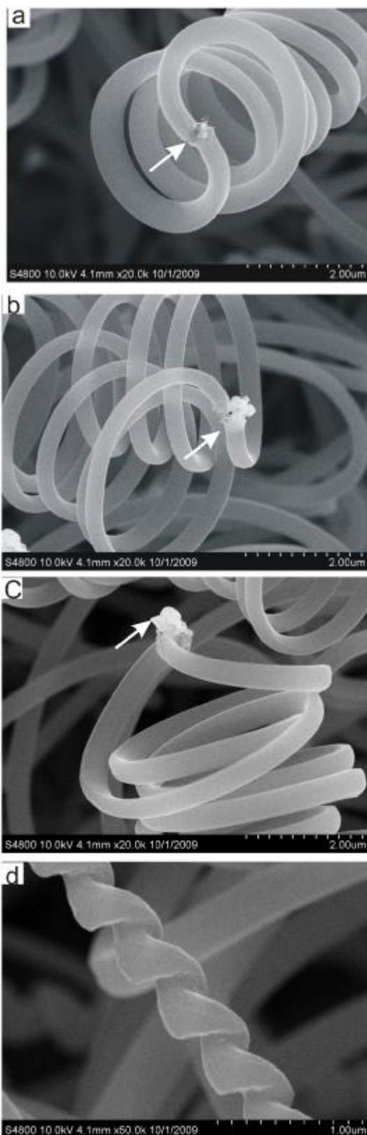
Fig.3 The growth tip morphology of spring-like double-helix microcoils (a,b and c) and morphology of twisting single-helix micocoils (d). The white arrows in (a), (b) and (c) indicate the nickel catalysts at the growth tip.
