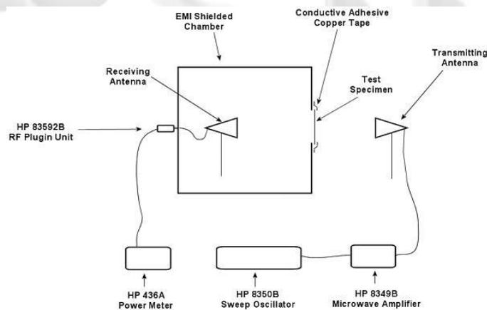
Figure 1. EMI Test fixture diagram
