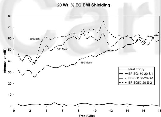
Figure 3. SE data versus 20 Wt. % of EG filler.
