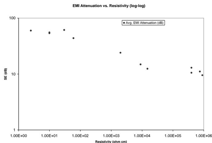
Figure 4. Log-log plot of EMI attenuation vs. resistivity. The sharp change in SE at low resistivity shows that a percolation threshold exists.
