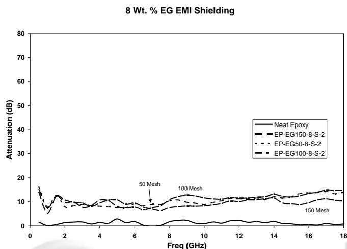
Figure 2. SE data versus 8 Wt. % of EG filler
