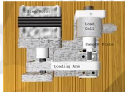
Fig . 2 Time Single fiber tension testing stage.
