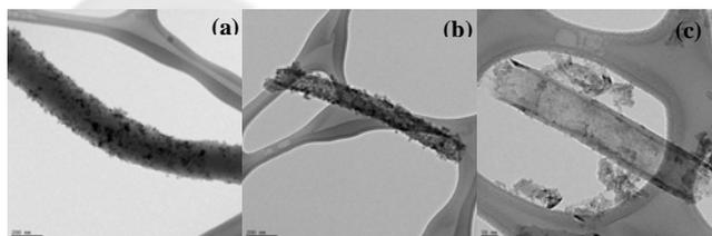
Fig. 2. TEM images of (a) TiO<sub>2</sub>/Gun-ei; (b) TiO<sub>2</sub>-Pyrograph; (c) TiO<sub>2</sub>-GANF
