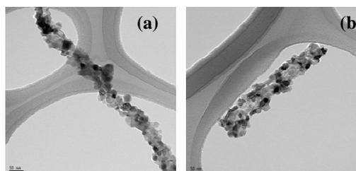
Fig. 3. Nanotubes of TiO<sub>2</sub> obtained from different CNF supports: a) Gun-ei and b) Pyrograph, after burning CNFs.
