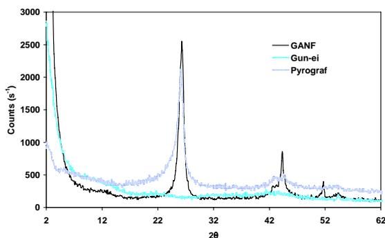
Fig.1. X-ray diffractograms of CNFs.
