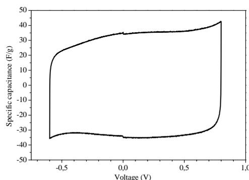
**Fig. 3** Cyclic voltammogram at a scan rate of  $10 \text{ mV}\cdot\text{s}^{-1}$  of TiC-CDC in 1M KOH electrolyte
