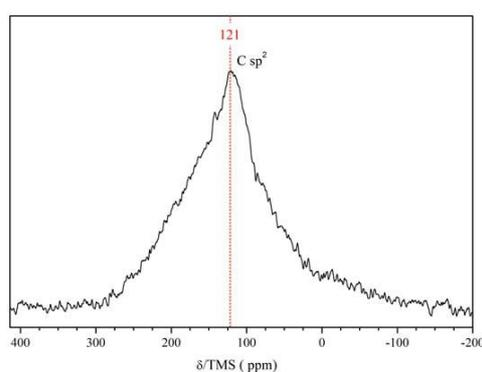
**Fig. 2** MAS  $^{13}\text{C}$ -NMR spectrum of titanium carbide after fluorination. The spinning rate is 10 kHz.
