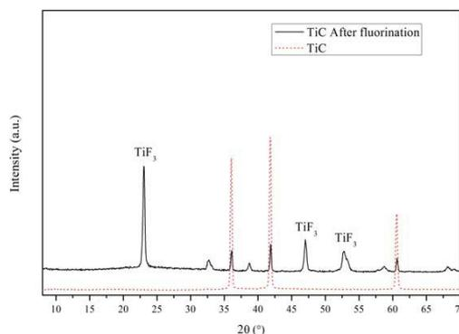
Fig. 1 XRD pattern of titanium carbide before and after fluorination
