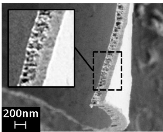
**Fig. 1** SEM images of SiC carbide after fluorination with  $\text{XeF}_2$ .
