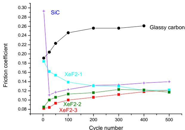
**Fig. 2** Friction coefficient evolution with the number of cycles of SiC thin films before and after fluorination with  $\text{XeF}_2$
