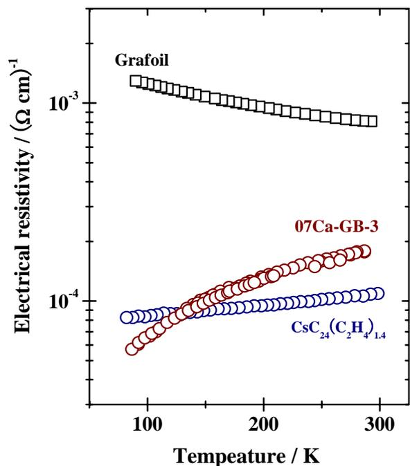
Fig.1 Temperature dependence in electrical resistivity of 07Ca-GB-3, Cs-ethylene-GIC and Grafoil.
