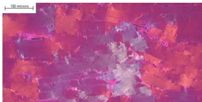
Fig. 2.1 Optical micrograph of carbonised composite
