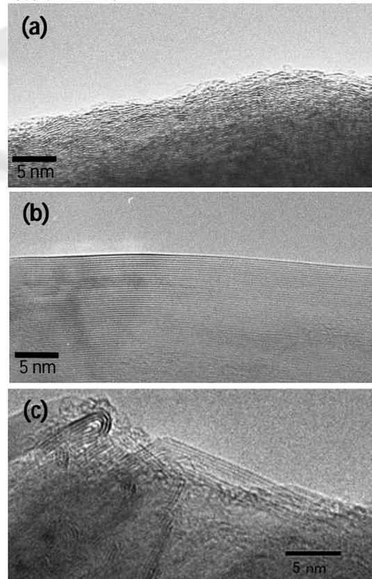
**Fig. 1** TEM observation: Typical carbon 002 lattice images of (a) CNS70p, (b) CNS70-26, and (c) CNS100-29.
