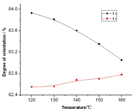
**Fig.4** The change of orientation degree with the temperature during the same period
