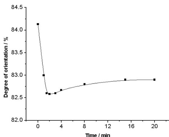
**Fig.3** The change of orientation degree with the thermal period at 140°C
