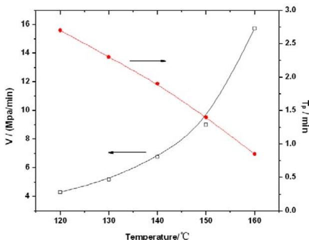
Fig.2 The climbing velocity ( $v$ ) and peak time ( $t_p$ ) of each process
