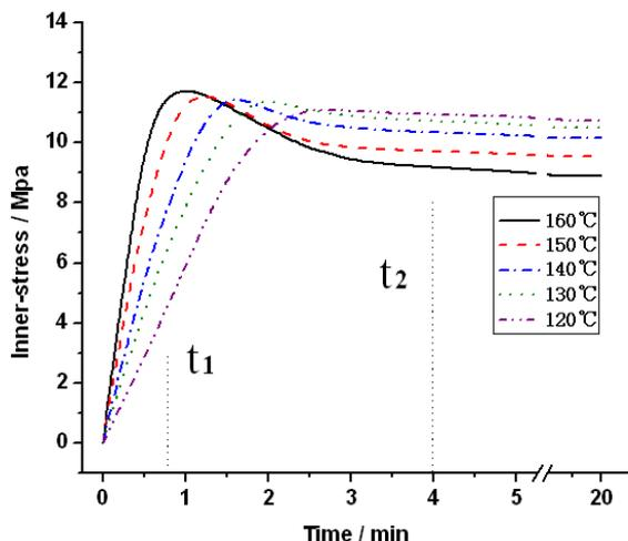
Fig.1 The relationship between inner-stress and heat treatment period
