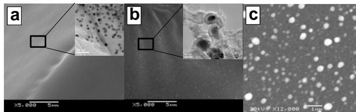
Fig. 1 SEM images of Ni/CFs obtained by carbonizing at (a) 700 °C, (b) 800 °C, and (c) 900 °C in flowing  $\text{N}_2$ .
