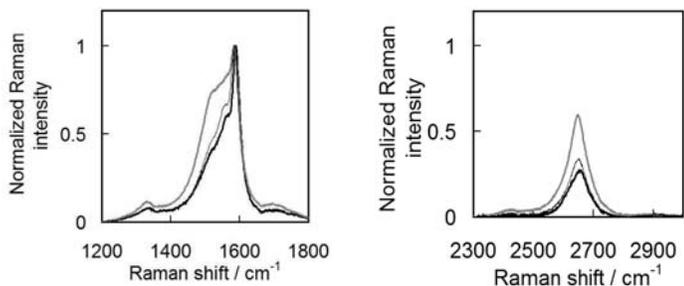
**Fig. 2** Raman spectra of SWCNTs before and after separation. Bold gray line: metallic SWCNTs, Bold black line: semiconducting SWCNTs, Thin line: SWCNTs before separation
