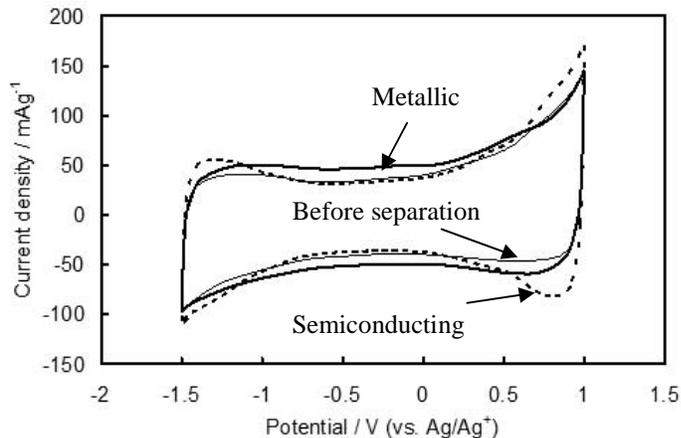
**Fig. 3** CVs of SWCNTs before and after separation. The curves were recorded at scan rate of 1 mV s<sup>-1</sup> in 1M TEABF<sub>4</sub>/PC.
