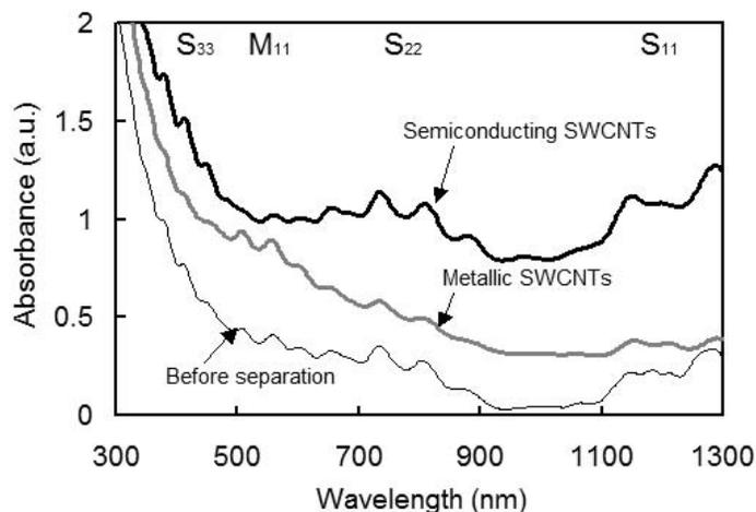
Fig. 1 SWCNTs before and after separation analyzed by UV-vis spectrometry.
