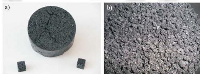
**Fig. 2** a) Cutted pieces from green coke column, b) Pseudo-needle shaped coke grains from chopped fibers
