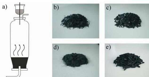
**Fig. 1** a) Coker drum / autoclave fiber dosing unit setup, b) PAN based chopped fibers, c) Pitch based chopped fibers, d) milled fibers, e) with epoxy resin pelletized milled fibers
