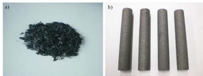
**Fig. 3** a) Shredded CFRP, b) extruded graphite rods
