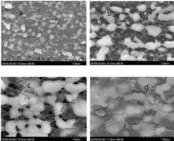
Fig. 4 SEM of coating fiber after heat treatment at 1600°C
