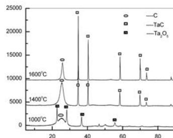
Fig.2 XRD patterns of the coating fibers after heat treatment at different temperature
