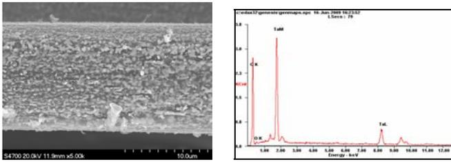
Fig. 3 SEM photos and EDS of coated fiber after heat treatment at 1600°C
