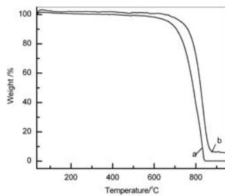
Fig.6 TGA of un-coated carbon fibers and TaC coated fibers
