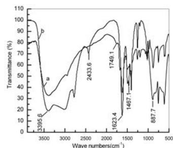
Fig. 1 FT-IR spectrum of precursor sol-gel of Ta
