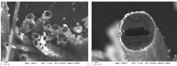
Fig. 5 Backscatter SEM of coating fiber after heat treatment at 1600°C
