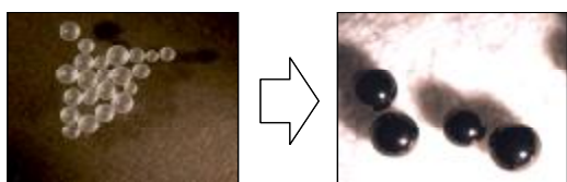
Picture 1: Cross linked polymer (left), PBSAC (right)
