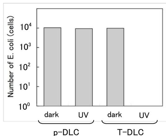
**Fig. 4** The antibacterial test results: the number of viable *E. coli* after 3 h staying in a darkroom (dark) and ultraviolet light irradiation (UV) of 3 h.
