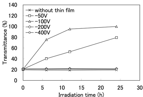
**Fig. 3** The measurement results of transmittances as for the DLC thin films deposited with bias voltages of -50 V to -400 V as a function of ultraviolet light irradiation time.
