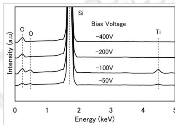
Fig. 1 The EDS analysis results for the DLC thin films deposited at the bias voltages of -50 to -400 V.
