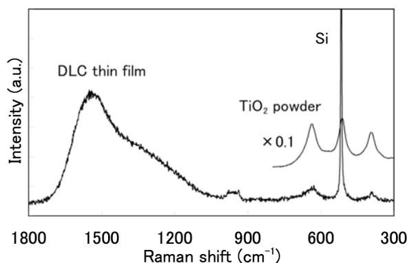
Fig. 2 The raman spectra for the DLC thin film deposited at bias voltage of -100 V and TiO<sub>2</sub> powder.
