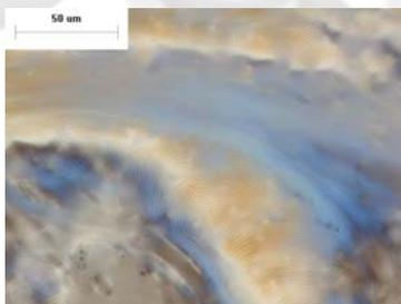
**Fig. 4** 2.32 vol% SWNTs under cross-polarized light. The scale bar is 50  $\mu\text{m}$ .
