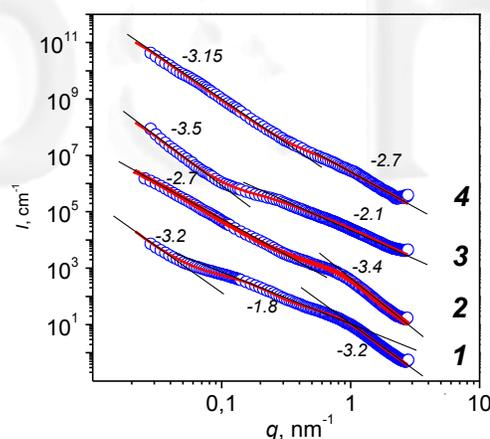
Fig. 2 Normalized SAXS curves in log(I) – log(q) scale: 1 – initial TC; 2 – 1.25% Ni on TC; 3 – 2.5% Ni on TC; 4 – 5.0% Ni on TC
