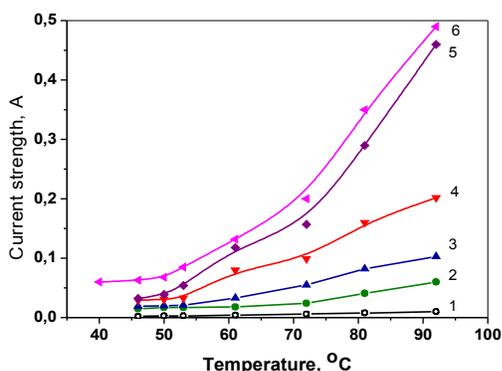
**Fig. 4** Current strength with temperature for different cathodes (U=12V): 1 – initial TC; 2 – 5.0%Ni/TC; 3 – 1.25% Ni/TC; 4 – 2.5% Ni/TC; 5 – Raney nickel; 6 – Palladium black.
