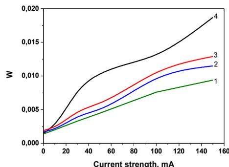
**Fig. 5** Isopropyl benzene hydrocracking rate: 1 – 5.0%Ni/TC; 2 – 1.25%Ni/TC; 3 – 2.5%Ni/TC; 4 – industrial Al-Ni-Mo catalyst.
