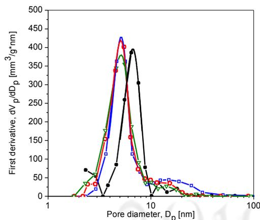
Fig. 1 Pore size distribution of TC with deposited Ni: 1 – initial TC; 2 – 1.25% Ni on TC; 3 – 2.5% Ni on TC; 4 – 5.0% Ni on TC.
