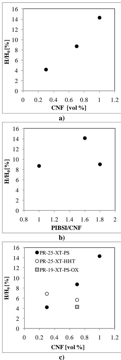
**Fig. 2** Percent improvement of the convection coefficient ( $h$ ) for the measured nanofluids as a function of a) fiber concentration, b) dispersing agent / fiber ratio concentration and c) fiber type and concentration.
