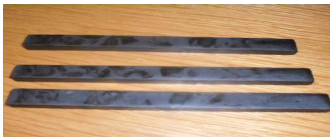
Fig. 1 Image showing injection molded coke pitch PVC test bars.
